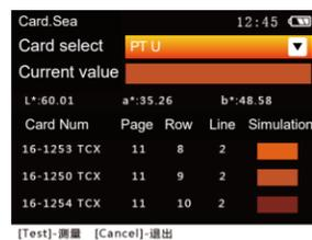
To improve the utility and convenience of our instrument, we develop spectrophotometer with build-in PT colors watches. After measurement, instrument can help us find three similar colors from the color swatches which can greatly improve working efficiency.
