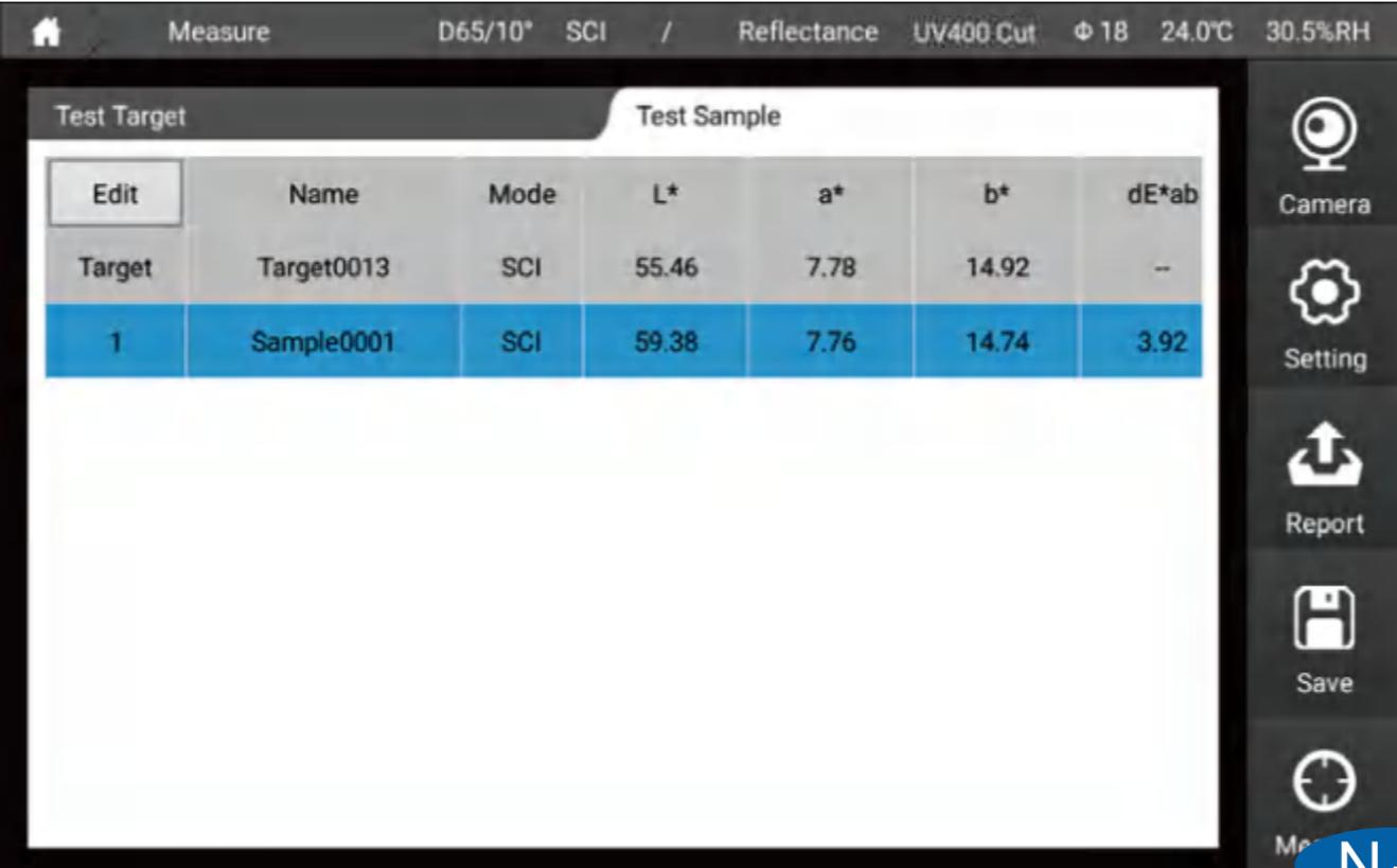
The screenshot shows a mobile application interface for color measurement. At the top, it displays 'Measure' and various settings: 'D65/10° SCI / Reflectance UV400 Cut Φ 18 24.0°C 30.5%RH'. Below this, there are two tabs: 'Test Target' and 'Test Sample'. The 'Test Sample' tab is active, showing a table with the following data:
