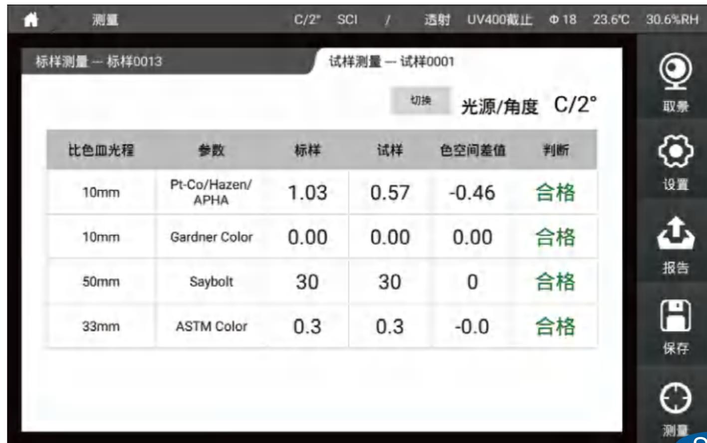
The screenshot shows the instrument's interface with a table of measurement results. The table has six columns: '比色皿光程' (Cuvette Path Length), '参数' (Parameter), '标样' (Reference), '试样' (Sample), '色空间差值' (Color Space Difference), and '判断' (Judgment). The data is as follows:
