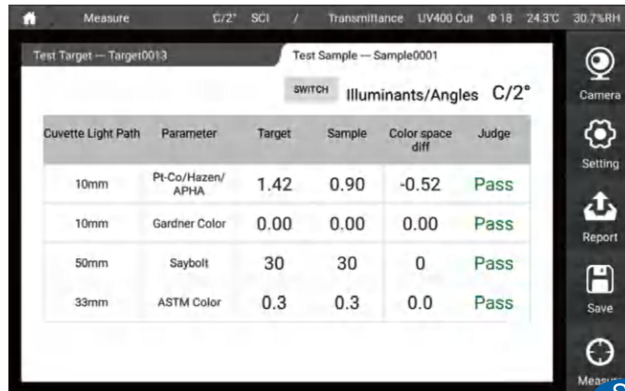
The screenshot shows the 'Measure' screen of a color instrument. At the top, it displays 'C/2° SCI / Transmittance UV400 Cut Φ 18 24.3°C 30.7%RH'. Below this, there are tabs for 'Test Target -- Target0013' and 'Test Sample -- Sample0001'. A 'SWITCH' button is set to 'Illuminants/Angles C/2°'. The main display is a table with the following data:
